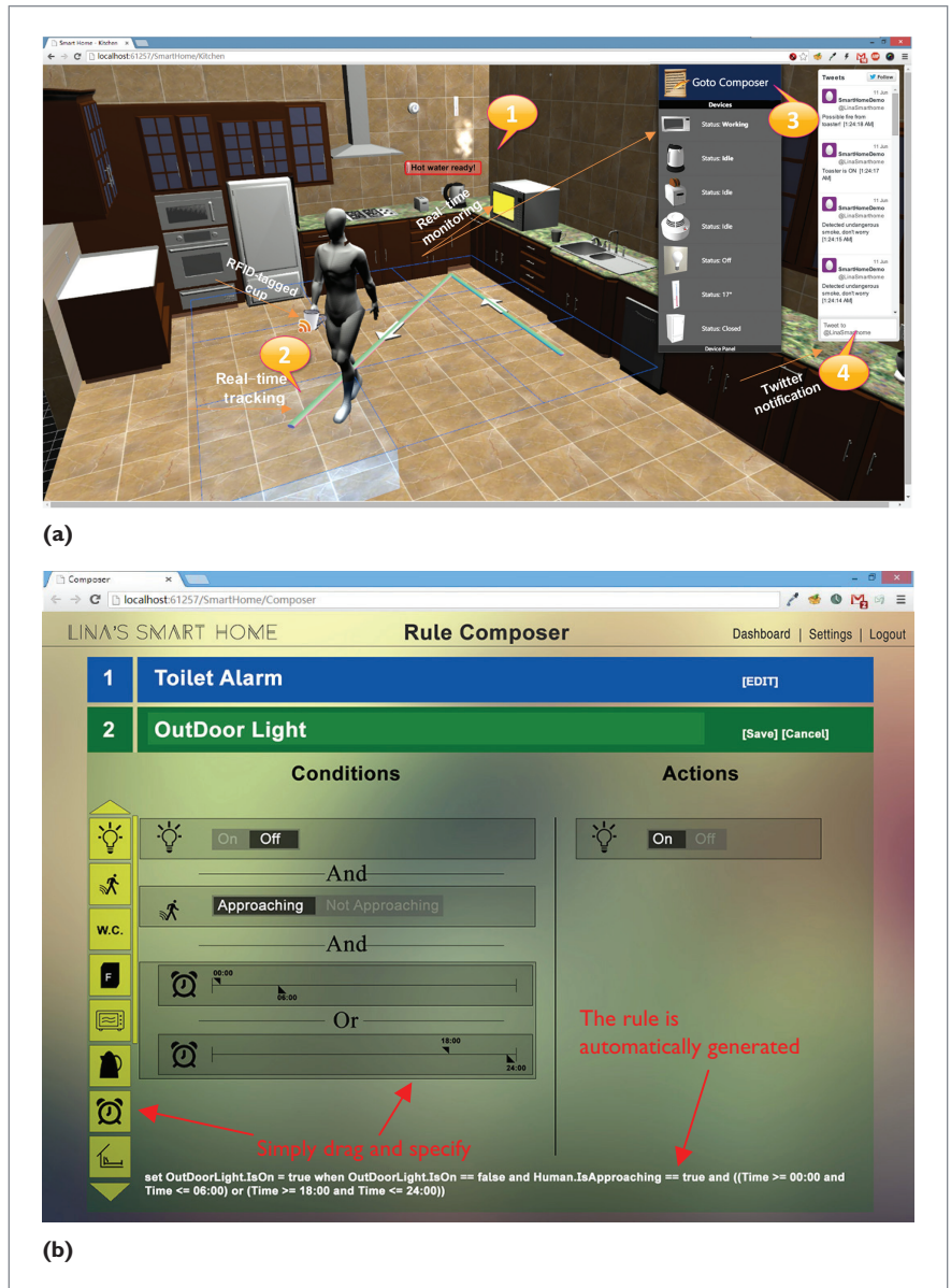
Figure 3. Real-time notification of things' status using Twitter. (a) The 3D Web-based application interface. (b) The rule composer supports users so that they can easily create their own rules. For example, for editing a rule like "turn on the outdoor light when a person is approaching during midnight to 6 am or 6 pm to midnight," a user needs only to drag the person and clock icons to the condition subpanel and the light icon to the action subpanel, and perform some simple adjustments (such as adjusting the clock slider to set the time period).
